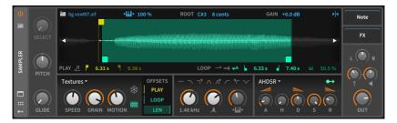
When only one audio file is loaded into the instrument, all relevant parameters appear within this section.
