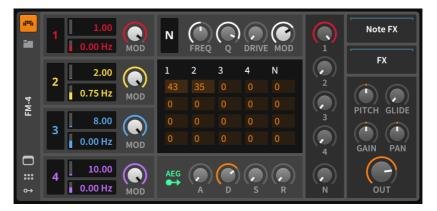
On the far left are four identically equipped sections, representing the four sine oscillator units of the instrument. Oscillator 1 is at top, oscillators 2 and 3 follow, and oscillator 4 is at bottom.
