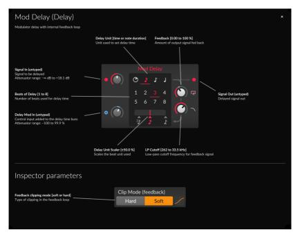
On the surface level, the help view displays all relevant parameter information for this type of module. In addition to the module's regular interface, any *Inspector parameters* are also shown below. This can be especially helpful as these parameters are often out of sight, out of mind.
