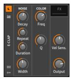
The *NOISE* section comprises the instrument's sound generation parameters. The amplitude for the instrument is controlled by an AD envelope that has a short, fixed attack time and an exponential, adjustable *Decay* time.
