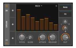
The drawbars section contains nine standard gain faders (the vertically higher the fader, the louder the gain), each of which represents the level of the respective drawbar harmonic. In order, these harmonics are:
