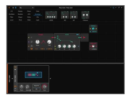
The result, shown above, is that **AR** has indeed been swapped out with **ADSR**. This includes any compatible parameters being maintained, all relevant patch cords being recreated, and all modulator paths being remapped to/from the new module.
