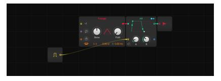
On the Triangle module, there is an arrow icon to the right of the yellow retrigger in port. This is a pre-cord for bringing all note gate signals reaching the device to the oscillator's retrigger port (for restarting the oscillator's phase). This toggle is disabled by default. Manually creating this connection would also require the Gate In module.
