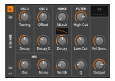
The OSC 1 section houses the primary sine oscillator, whose frequency and decay time can be set directly with the *Tuning* and *Decay* knobs, respectively.
