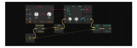
To make a feedback connection: insert a **Long Delay** (*Delay/FX*) module into the feedback path.
