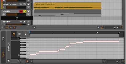
On this new instrument track, a **Sampler** device has also been created with the corresponding slice of audio assigned to each note seen in the note clip.
