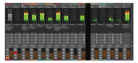
The send section is the block of right-aligned knobs beneath the device section. In the image above, there are four FX tracks present, with corresponding send knobs on each track. These sends allow us to pass a portion of each track's audio into the various FX tracks. Using a send does not affect a track's main output level.
