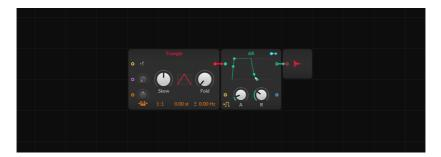
> On the AR module, there is an icon in the bottom left corner representing a two-state logic signal. This is a pre-cord for bringing all note gate signals reaching the device to the envelope generator's gate in port. This toggle is enabled by default as envelope generators are most often gated by note input. Manually creating this connection would require the Gate In module.
