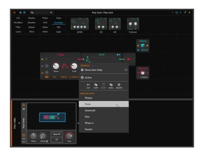
Both methods of replace would produce the exact same outcome — in this case, a **Pulse** oscillator in place of the **Triangle** oscillator, using any corresponding settings and the connections that the original had.
